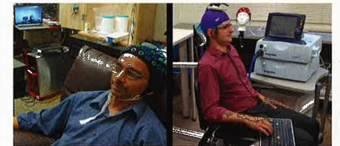
MEETING OF MINDS: Researcher Rajesh Rao (left) imagines firing a weapon in a video game. His neural signals are picked up by cap electrodes and transmitted via Internet to Andrea Stocco (right) across campus. Stocco's cap turns the signal into a magnetic pulse, causing him to press the "fire" button.
