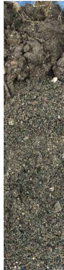
Figure 2. Three inches of topsoil fill, on top of sand deposits from Bozeman Creek
