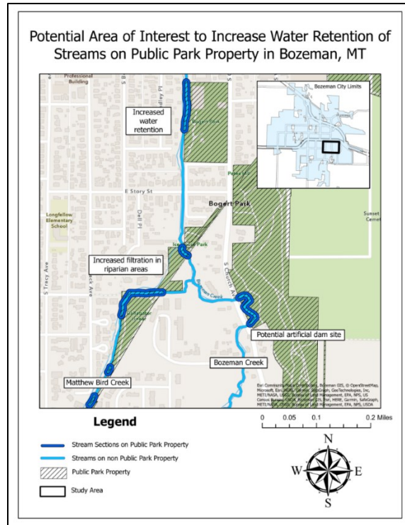
Figure 3: Potential area to implement retention/detention management practices on stream paths in public parks. Proposed approaches provide increased scope for natural filtration and storage.
